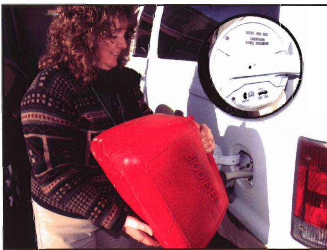
Figure 1.3. Biodiesel can be poured directly into fuel tanks of newer vehicles that run on diesel fuel with no modification to the engine nor fuel system.
