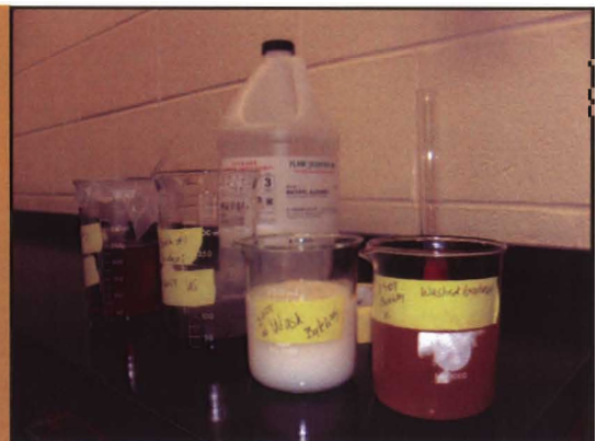
Figure 3.17. Ms. Schmieder drains the parts that have separated and labels them "washed biodiesel" (foreground) and "glycerin" (background).
