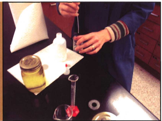
Figure 3.7. She adds two drops of phenolphthalein, a pH indicator.
