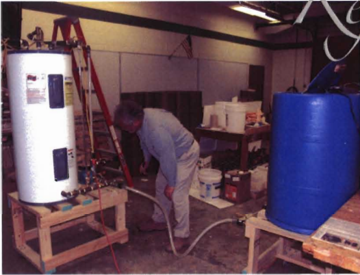
Figure 3.28. Mr. Bullock checks the functionality and direction of fluid flow of the pump to the wash tank.
