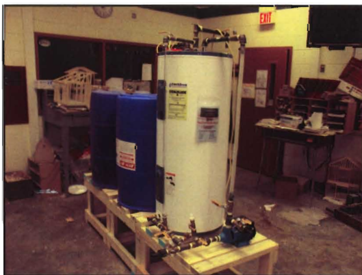
Figure 3.22. Student built wooden stands with casters from Internet plans to enable the wash tanks (blue containers) to be positioned along side of the refinery.
