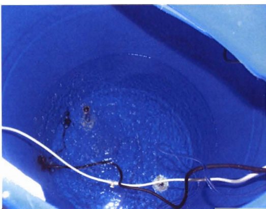
Figure 3.27. A bubbling and misting system cleans unwashed biodiesel and then it is allowed to dry by air or heating to evaporate the water.
