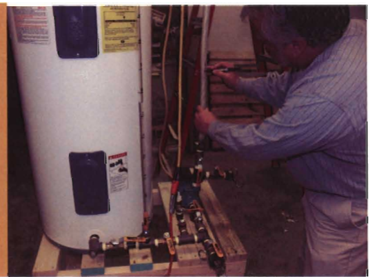
Figure 3.29. He then marks the direction of flow on a previously calibrated plastic tube.
