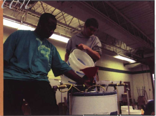
Figure 3.24. Students pour tap water into the refinery to check its capacity and look for plumbing leaks.
