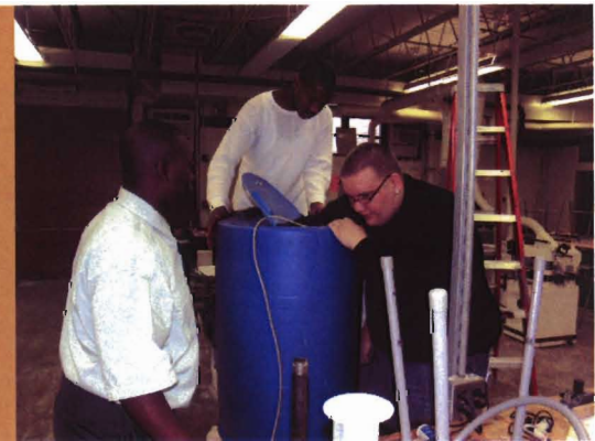
Figure 3.26. Students assemble an integral part of the biodiesel refining process: the wash tank. When biodiesel is separated from glycerin, it is cloudy from impurities.
